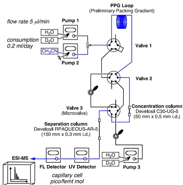
**Figure 2.** Example of house-assembled flow system equipped with PPG (pre-packed gradient), capillary UV, FL-detectors, into ESI-Q-TOF-MS.
